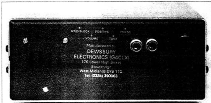
Fig. 2 Rear view showing keying sockets for solid state and valve rigs, together with headphone jack. The two holes at the bottom right give access to presets to adjust sidetone pitch and volume.
