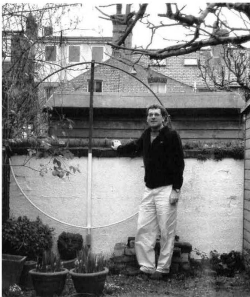
Fig 3: The author with the completed 1.8MHz receiving loop in its final setting with its low-profile camouflage colour scheme!
